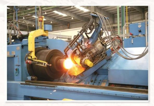
The tube is taken for the bottom spinning process where one end of the seamless tube is heated in the Induction furnace up to 1200° C & then fed into the high speed CNC operated Hot Spinning Machine to get desired bottom shape. The world class German machines 'Leifeld' installed at our plant ensure that the cylinder fusion takes place at the center, joints are leak free and that proper dimensional tolerances and dome shape is maintained at all times.
