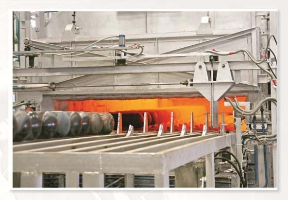
The cylinder is processed through a LPG fired heat treatment furnace which is one of the best technologies available in the world to ensure proper strength of material. The hardening, quenching & tempering operations are done at continuous walking beam type furnace with maintenance of proper concentration of polymer quenchant shell.
