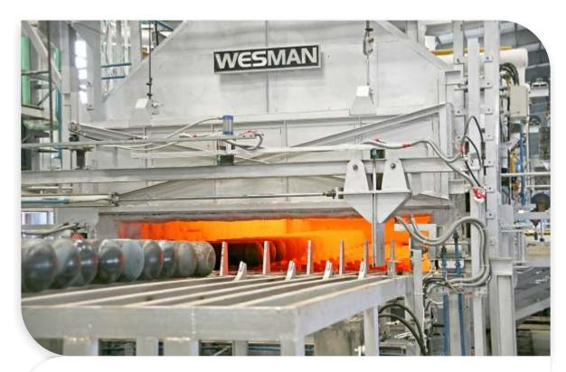
The cylinder is processed through a LPG fired heat treatment furnace 'Wesman' to ensure proper strength of material. The hardening, quenching & tempering operations are done at continuous walking beam type furnace with maintenance of proper concentration of polymer quenchant shell. The proper Temperatures maintained at various levels are as follows:-
