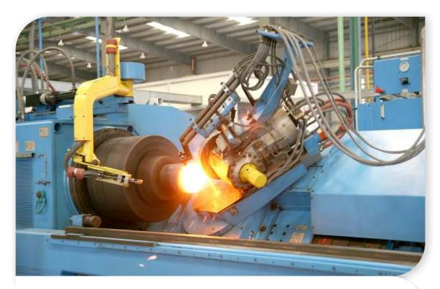
The tube is taken for the bottom spinning process where one end of the seamless tube is heated in the Induction furnace up to  $1200^{\circ}$  C & then fed into the high speed CNC operated Hot Spinning Machine to get desired bottom shape. The world class German machines 'Leifeld' installed at our plant ensure that the cylinder fusion takes place at the centre, joints are leak free and that proper dimensional tolerances and dome shape is maintained at all times.
